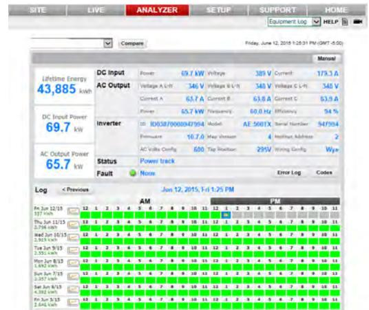
Fig 14 Detect intermittent internet connection from weak cellular or down land lines with the 30 day Communication log
